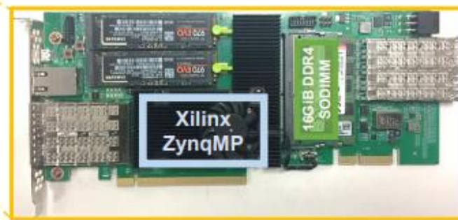
Custom FPGA Board with a Xilinx Zynq UltraScale+ MPSoC (ZynqMP) Chip
