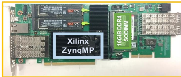
Custom FPGA Board with a Xilinx Zynq UltraScale+ MPSoC (ZynqMP) Chip
